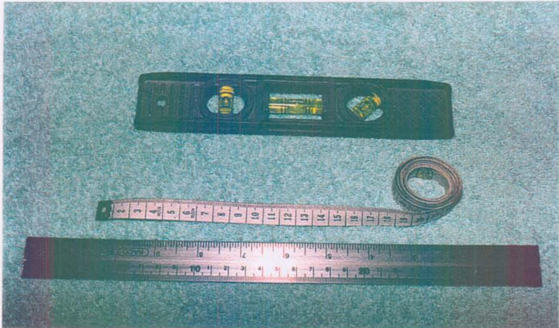
Figure 3: Measuring tape, spirit level and metal ruler
